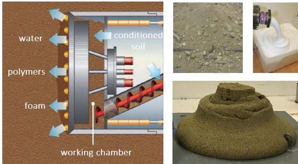
Figure 1. EPB-TBM scheme on the left and laboratory soil conditioning process on the right.
