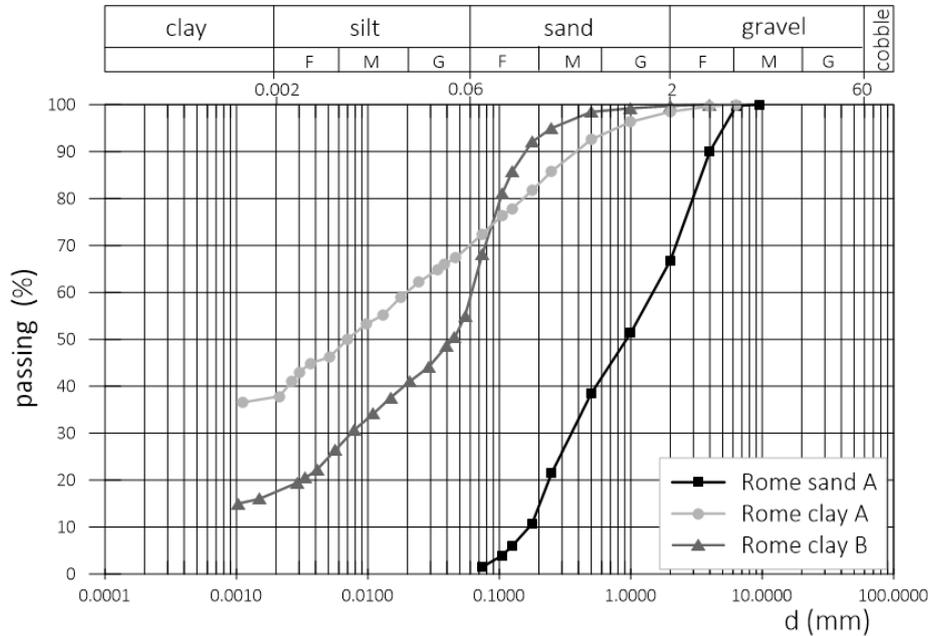
Figure 3. Grain size distribution of Rome sand A, Rome clay A and Rome clay B.
