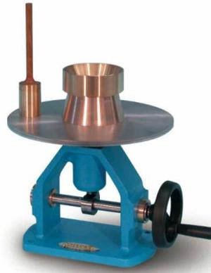
Figure 2. Flow table test apparatus.
