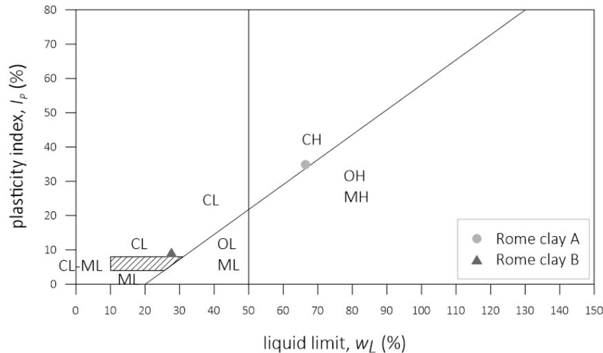
Figure 4. Casagrande plasticity chart of Rome clay A and Rome clay B.
