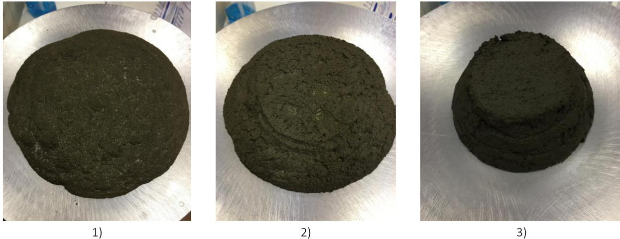
Figure 6. Results after 40 drops for: 1) over-conditioned Rome clay A, 2) over-conditioned Rome clay A treated with 5% of Porous Alpha; 3) over-conditioned Rome clay A treated with 27% of Porous Alpha.
